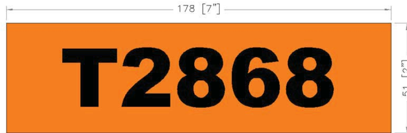
Figure-8 Transformer Identification Label (Example)
