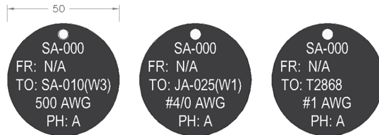
Figure-5 Primary Cable Identification Tags (Example)
